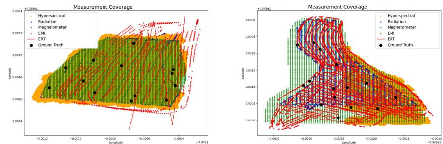
Figure 1: Sensor measurement points and ground sample locations across Site 1 (left) and Site 2 (right). Gaps in hyperspectral data (e.g., west side of Site 2) and limited spatial coverage for EMI and radiation sensors are visible.
